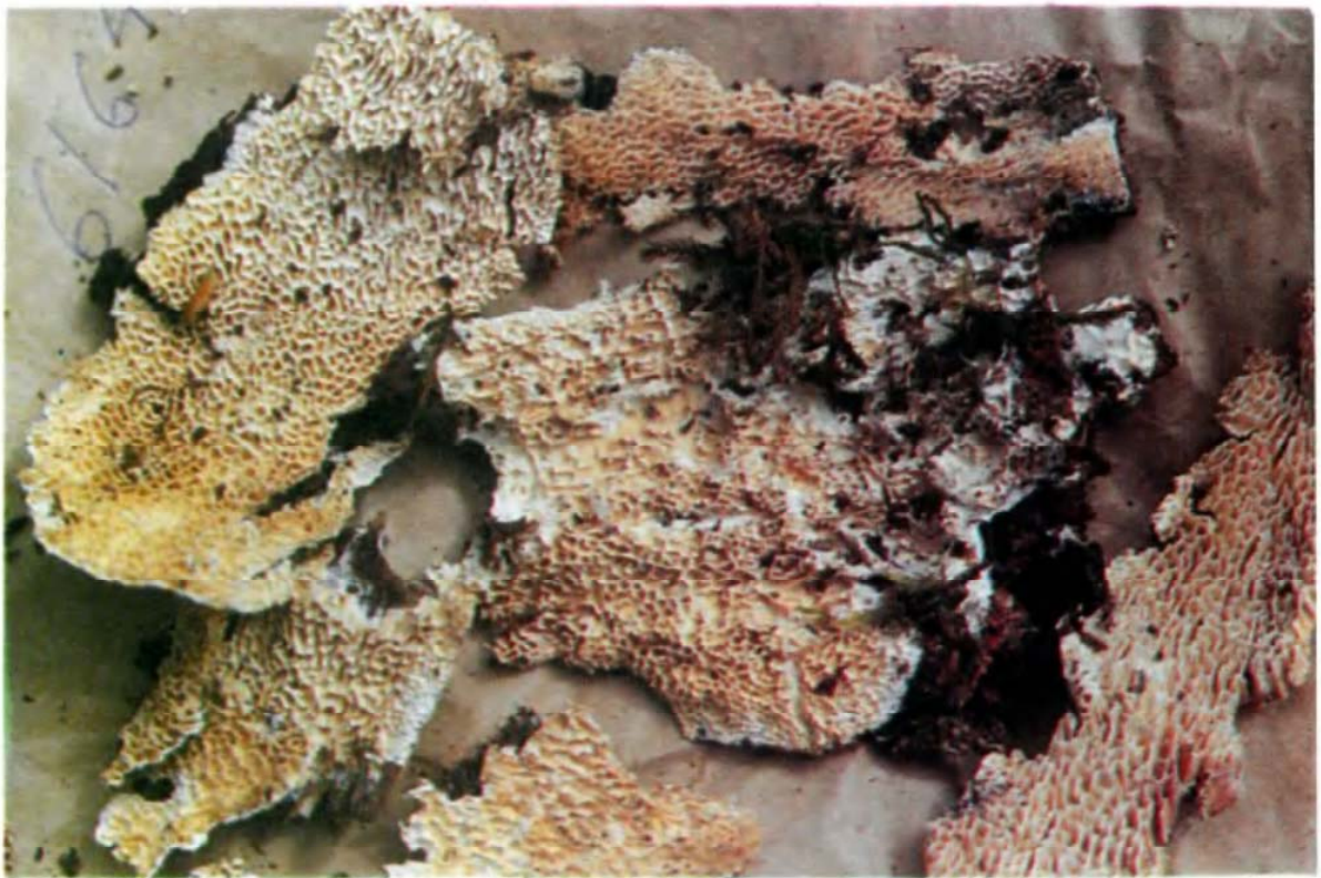
Fig. 5. Antrodia albida (Fr. : Fr.) Donk growing frequently on structural coniferous timber and causing brown rot.
